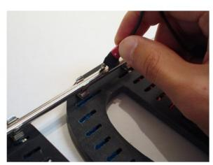
H2. Attach the red clip terminal to the top Stainless Steel Rod. For a professional look attempt to obscure clip terminals beside a bracket or behind a round and closed letter, number, or symbol.
