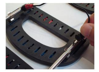
H3. Attach the black clip terminal to the bottom Stainless Steel Rod.
