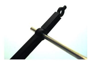
D4. Align and carefully insert the Stainless Steel Rods into all of the holes of the Rod Brackets, leaving protrusions of about 1 inch.
